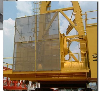
Mini Heatshields protecting Boom Hoist Control Point
